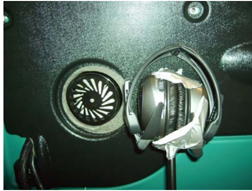
Figure 26 illustrates the active noise canceling headphones with a microphone embedded between the ear muffs
