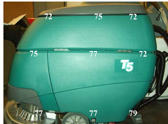
Figure 30 & 31 Sound maps for the left and right side of the floor scrubber with attached rubber seal (measured in dBA)
