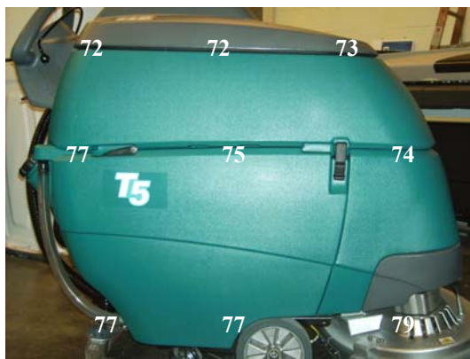
Figure 30 & 31 Sound maps for the left and right side of the floor scrubber with attached rubber seal (measured in dBA)
