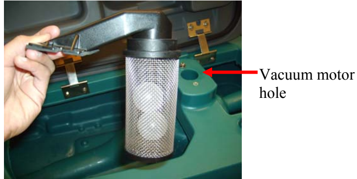
Figure 33 close up picture of the original elbow pipe design
