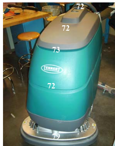
Figure 32 Sound map for the front and top of the floor scrubber with attached rubber seal (measured in dBA)
