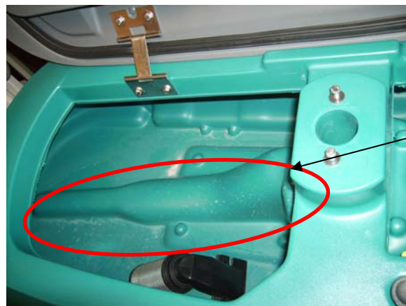
Figure 70 illustrates the current muffler indent that needs to be enlarged to accommodate the new design.
