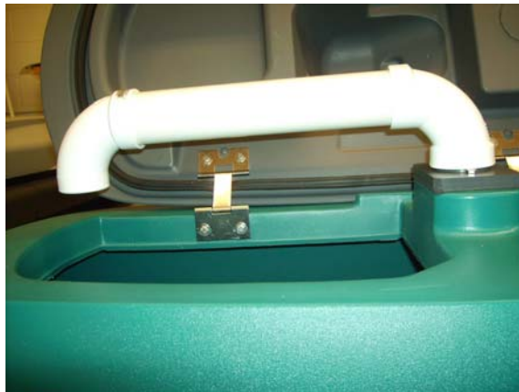
Figure 56 illustrates the elbow pipe prototype.
