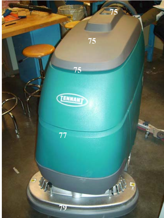
Figure 11 shows a Sound Map of the Front and Top of the floor scrubber with noise level in dBA.
