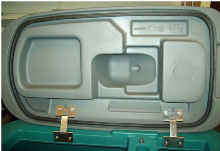
Figure 69 illustrates the current recovery tank lid that needs to be redesigned to accommodate the new elbow pipe.
